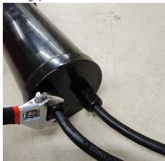
c. Pull the wires out of the top of the enclosure so that the terminals are accessible.
