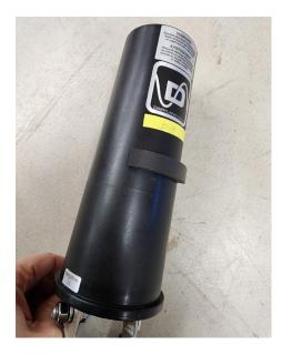
g. Push SSD/OVP2 as far down into the enclosure as it can go, continuing to feed the wires through the enclosure and out the cord grips at the bottom.
