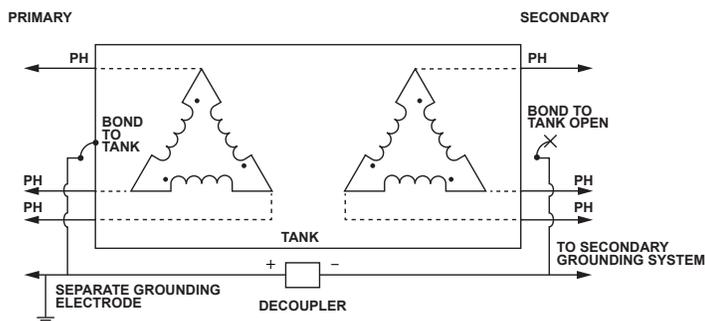
**11b.** With decoupler installed and CP current paths cleared
