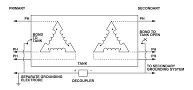
11b. With decoupler installed and CP current paths cleared
