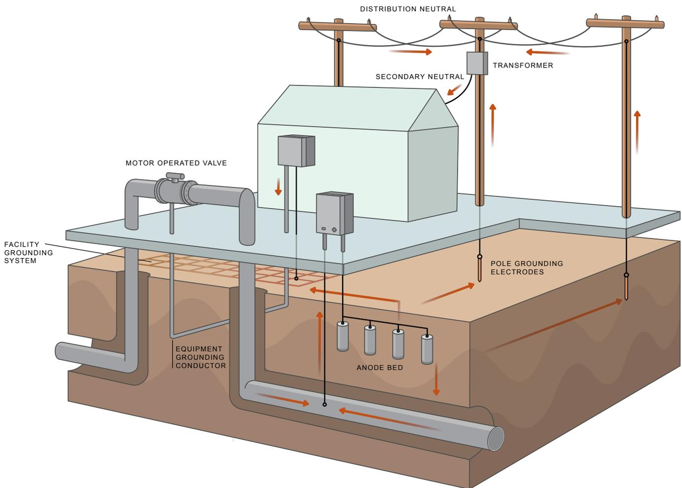
Figure 1. Facility cathodic protection interacts with power utility grounding system.
