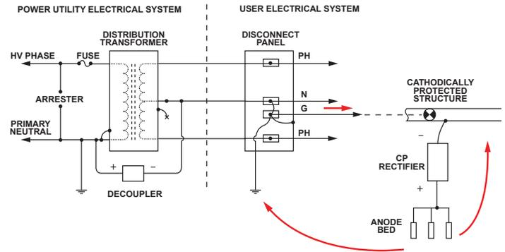
Figure 5. Effect of decoupling on typical electrical service involving cathodic protection.
