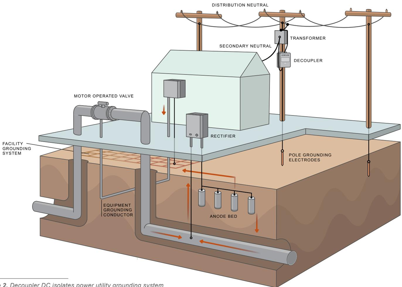
Figure 2. Decoupler DC isolates power utility grounding system
