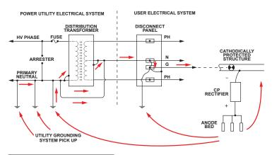
**Figure 4.** Current flow on typical electrical service involving cathodic protection.
