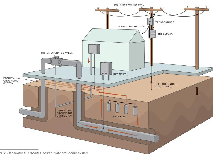
Figure 2. Decoupler DC isolates power utility grounding system
