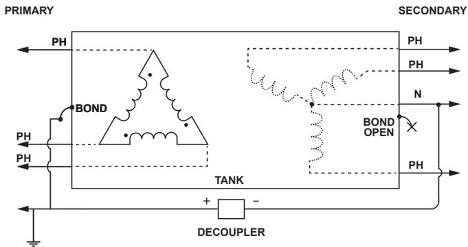
9b. With decoupler installed and CP current paths cleared
