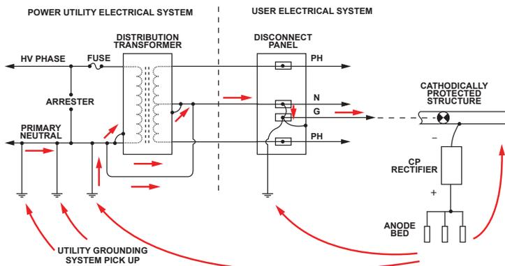
Figure 4. Current flow on typical electrical service involving cathodic protection.
