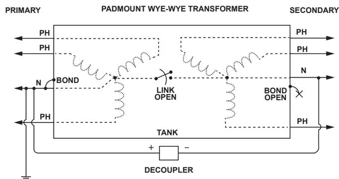
Figure 8. Decoupler installation at a three-phase Wye-Wye pad-mounted transformer.
