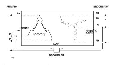
9b. With decoupler installed and CP current paths cleared
