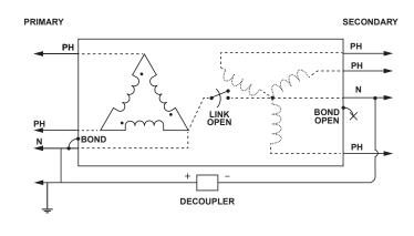
10b. With decoupler installed and CP current paths cleared
