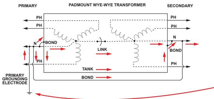
Figure 7. Three-phase pad-mounted transformer connections allowing CP current flow.
