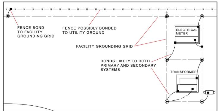
**Figure 12.** Site plan showing additional bonding between primary and secondary that allow CP bypass.
