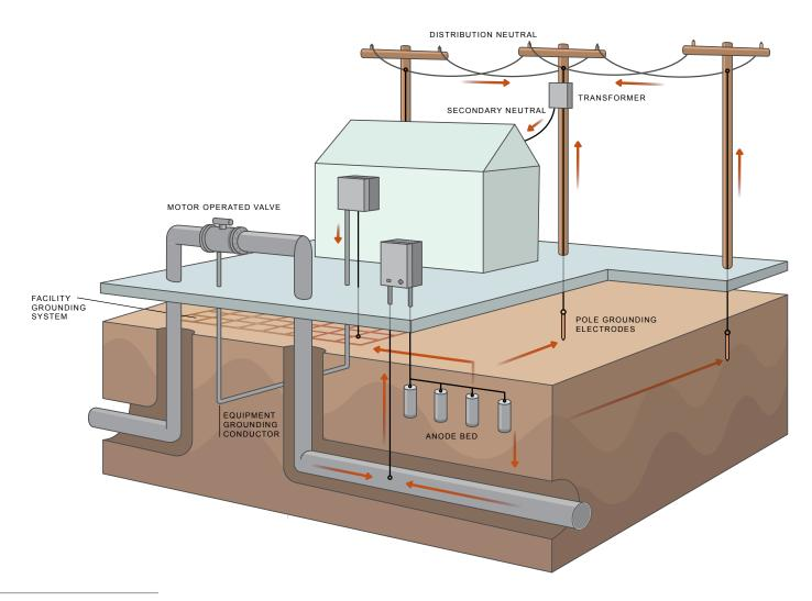
Figure 1. Facility cathodic protection interacts with power utility grounding system.
