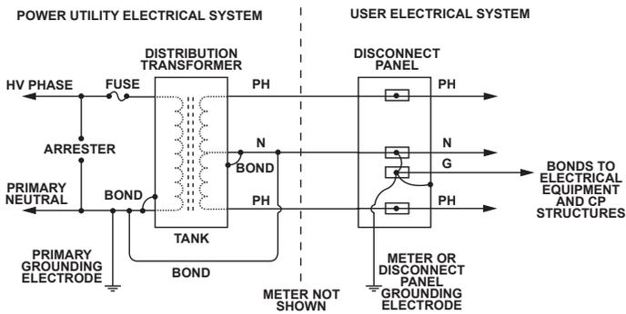
Figure 3. Typical electrical service involving cathodic protection.
