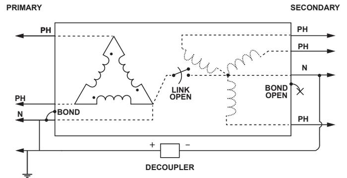
10b. With decoupler installed and CP current paths cleared
