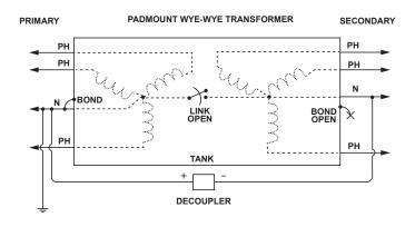
Figure 8. Decoupler installation at a three-phase Wye-Wye pad-mounted transformer.
