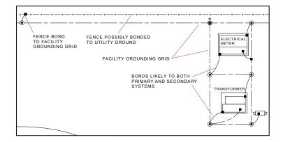
**Figure 12.** Site plan showing additional bonding between primary and secondary that allow CP bypass.
