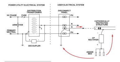
**Figure 5.** Effect of decoupling on typical electrical service involving cathodic protection.
