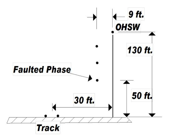
Figure F-7: Cross-Sectional Geometry of Transmission Line
