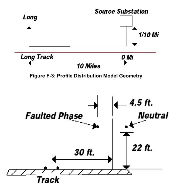
Figure F-4: Cross-Section Distribution Model Geometry
