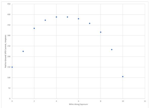
Figure L-8: Calculated Maximum Fault-Induced Current through Rail-to-Ground HEFPDs at non-IJ Locations
