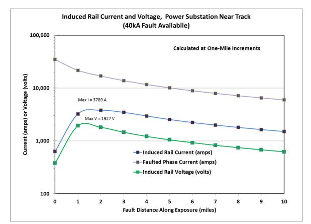
Figure F-8: Induced Rail Current and Voltage as a Function of the Transmission Line Fault Location
