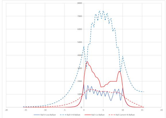
Figure L-5: Composite Calculated Maximum Rail Voltage and Current versus Fault Location Along Exposure for Low & High Values of Track Ballast Resistivity
