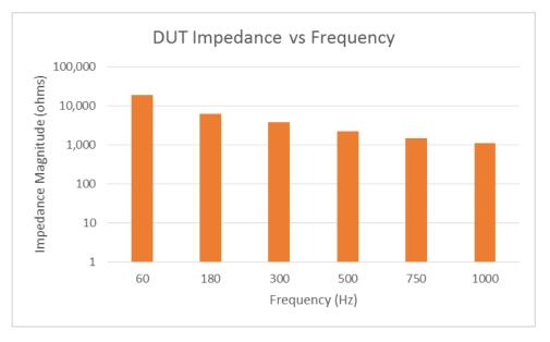
Figure H-2: Measured Impedance of Tested HEFPD.
