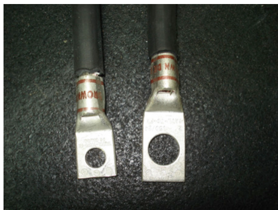
Terminal for 5/16" bolt (left), 1/2" bolt (right)
