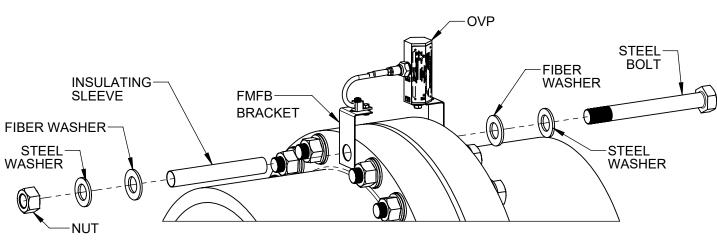
THE OVP SPECIFIC FMFB KIT CONSISTS OF (2) IDENTICAL NICKEL PLATED COPPER BRACKETS, THE REQUIRED ASSEMBLY HARDWARE, AND CORROSION INHIBITOR (TEFGEL) FOR MOUNTING ANY OVP MODEL PRODUCT TO AN INSULATED FLANGE OF THE BOLT HOLE DIAMETER (OR ANSI # CLASS AND PIPE DIAMETER) FOR WHICH IT WAS ORDERED.
