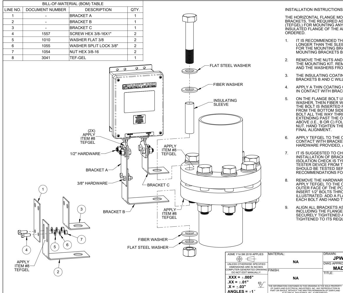
THE HORIZONTAL FLANGE MOUNT KIT CONSISTS OF (3) NICKEL PLATED COPPER BRACKETS, THE REQUIRED ASSEMBLY HARDWARE AND CORROSION INHIBITOR (TEFGEL) FOR MOUNTING ANY PCR MODEL WITH STANDARD TERMINALS TO AN ÎNSULATED FLANGE OF THE ANSI # CLASS AND PIPE DIAMETER FOR WHICH IT WAS ORDERED.
