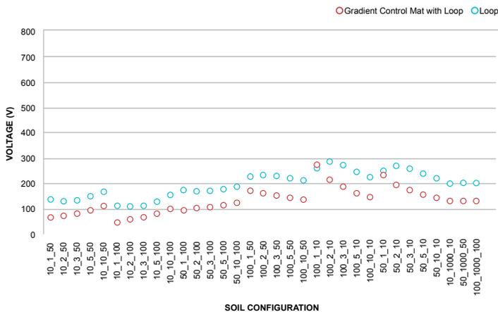
Figure 8 – Dairyland Gradient Control Mat Step Voltages for Grounding Loop on Mat Placed at 600MM Depth
