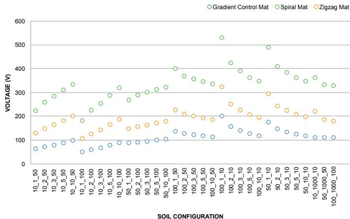
Figure 2 – Touch Voltage for Mat Placed at 600MM Depth
