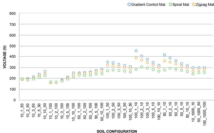
Figure 6 – Step Voltages for One Foot On and One Foot Off Mat Placed at 600MM Depth
