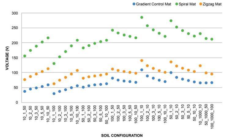
Figure 3 – Step Voltages for Both Feet on Mat Placed at 150MM Depth
