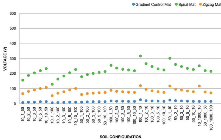
Figure 1 - Touch Voltage for Mat Placed at 150MM Depth
