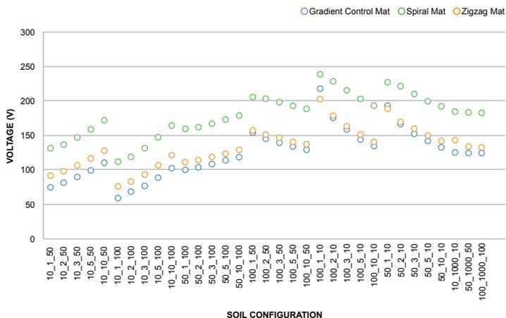
Figure 4 – Step Voltages for Both Feet on Mat Placed at 600MM Depth
