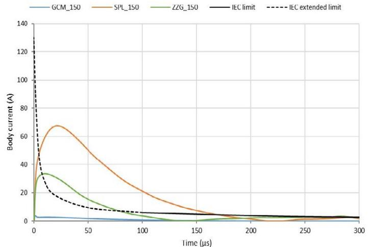
Figure 9 – Threshold Limits of Lightning Strike Causing Ventricular Fibrillation
