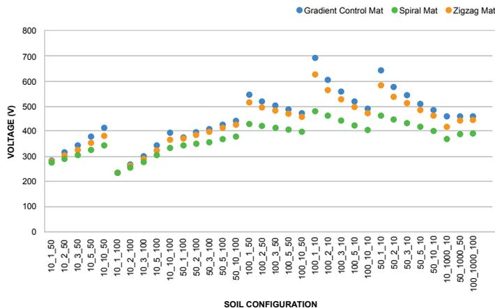
Figure 5 – Step Voltages for One Foot On and One Foot Off Mat Placed at 150MM Depth
