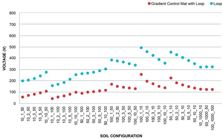
Figure 7 – Dairyland Gradient Control Mat Step Voltages for Grounding Loop on Mat Placed at 150MM Depth
