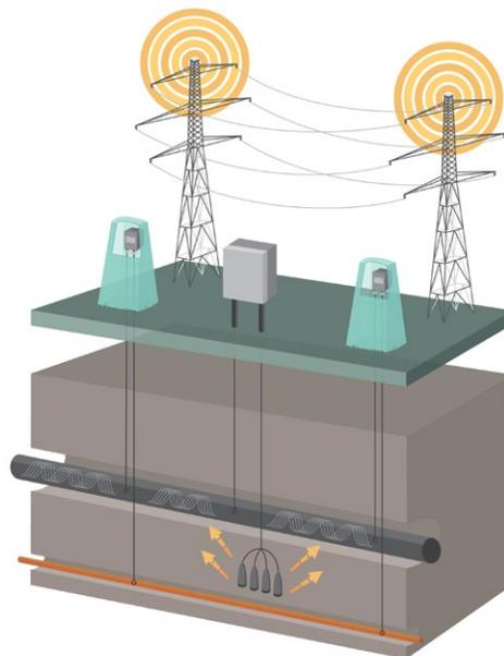
*Decoupled systems provide simultaneous AC grounding and DC isolation optimizing your CP system and simultaneously mitigating induced AC to your grounding system.*
