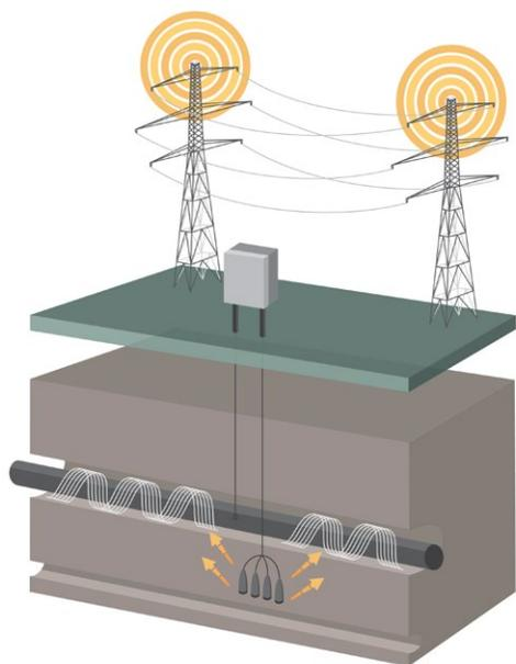
*Electric and magnetic fields can cause unwanted voltage to appear on nearby pipelines creating a safety risk and corrosion threat.*
