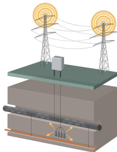
*Mitigation systems such as zinc ribbon direct bonded to address safety and corrosion risks from induced AC cause adverse affects on your CP system.*
